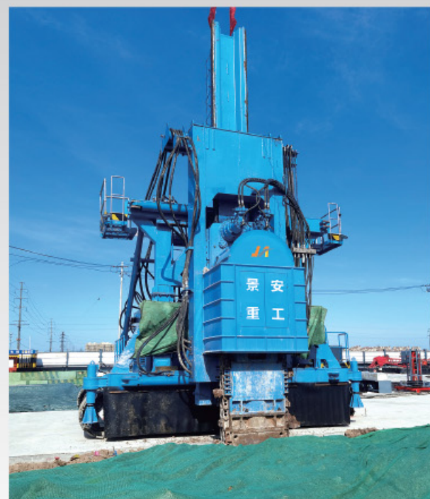
Qingdao Subway Width 900mm, Depth 45m Construction model: TRDE7095/TRD4585
