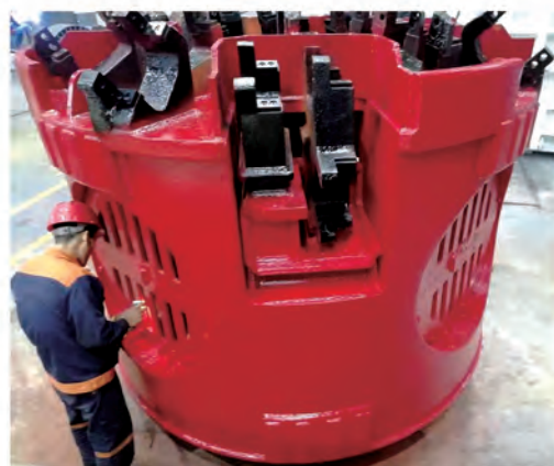
扩孔钻头，用于在钻进中扩大孔径 Reaming bit, used to enlarge the hole diameter in drilling
