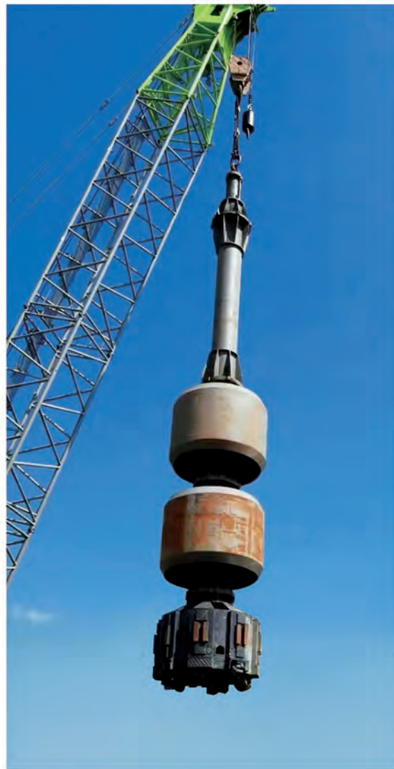
钻具组装总图 General assembly of drilling tool
