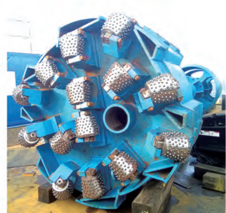
安装滚刀后的平钻头 Flat drill bit after installing hob
