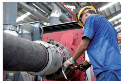
钻杆焊接前预热，焊后保温， 确保焊接可靠 Drill pipe shall be preheated before welding and insulated after welding to ensure reliable
